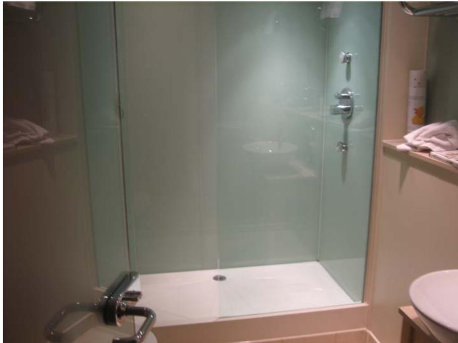
Door on the left, designed to prevent reaching the controls from the outside or shelves from the inside, and to reflect water into the room.
