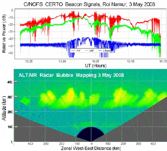
Figure 3. Comparison of radio wave scintillations at 150, 400, and 1067 MHz (top) with radar backscatter from field aligned irregularities (bottom).
