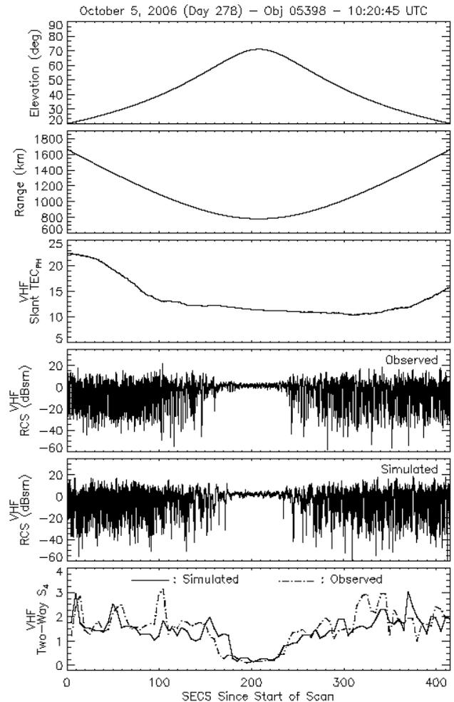
Figure 2. Apparent radar cross section of a spherical target observed through a structured equatorial ionosphere on 5 October 2006.
