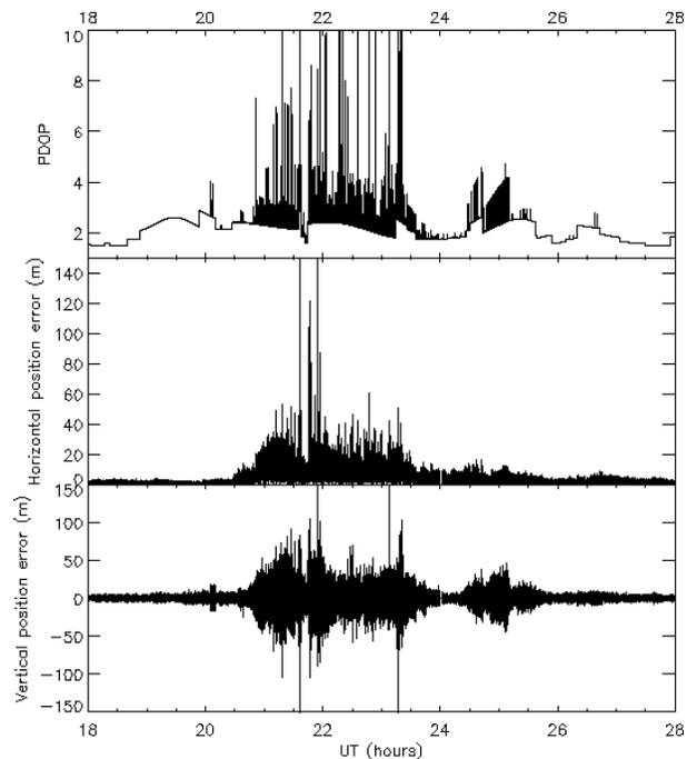
**Figure 7.** Simulated PDOP, simulated horizontal position error and simulated vertical position error versus time.
