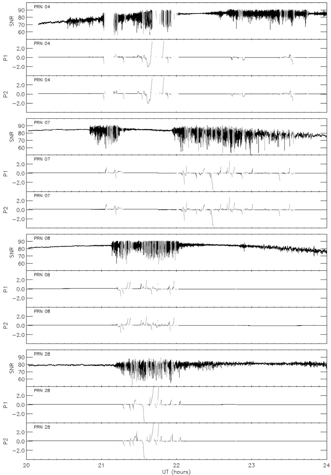
**Figure 5.** Signal-to-noise ratio on the L1 carrier (dB-Hz), and detrended L1 & L2 pseudoranges (km). The excursions from zero in the detrended pseudoranges are principally due to scintillation induced ranging errors. Black and gray indicate nominal and anomalous tracking status, respectively.
