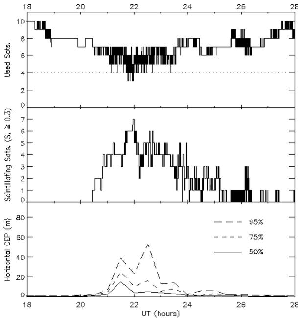
**Figure 1.** Time versus number of satellites used in the position solution (top), the number of scintillating satellites with  $S_4 \geq 0.3$  (middle) and the horizontal CEP at the 50<sup>th</sup>, 75<sup>th</sup> and 95<sup>th</sup> percentiles (bottom), based on a 30-minute moving window.
