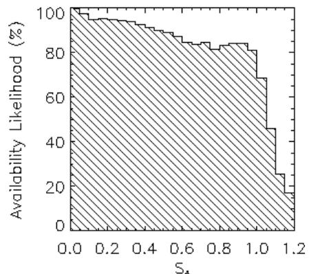
**Figure 3.** Histogram showing the likelihood of a link being included in the position solution versus the scintillation intensity on that link.
