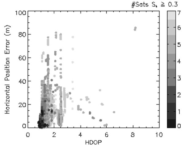
**Figure 4.** Horizontal position error versus horizontal dilution of precision. The points are colored by the number of scintillating satellite links with  $S_4 \geq 0.3$  at that time.
