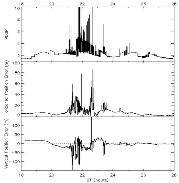
**Figure 2.** Time versus position dilution of precision (top), horizontal position error (middle), and vertical position error (bottom).
