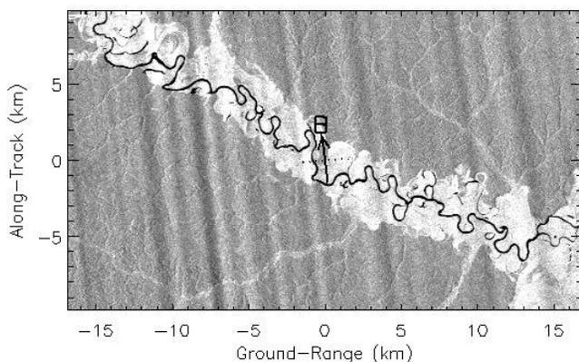
Figure 3. PALSAR sub-look on 26 March 2008 showing evidence of ionospheric streaking.
