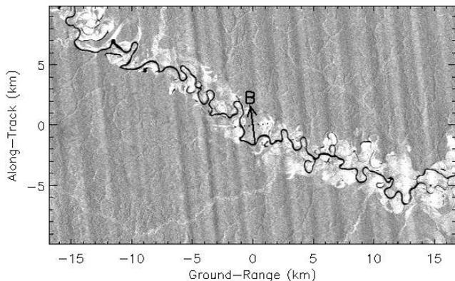
Figure 4. Simulated PALSAR observation obtained by imposing ionospheric effects on the image shown in Figure 2.
