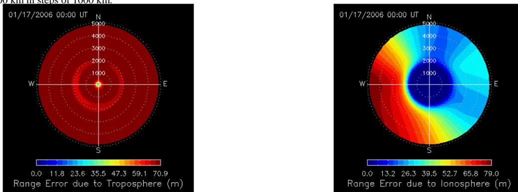
Fig. 3. An estimate of the separate contributions to range error of the troposphere (left panel) and the ionosphere (right panel) at an elevation of 1°.
