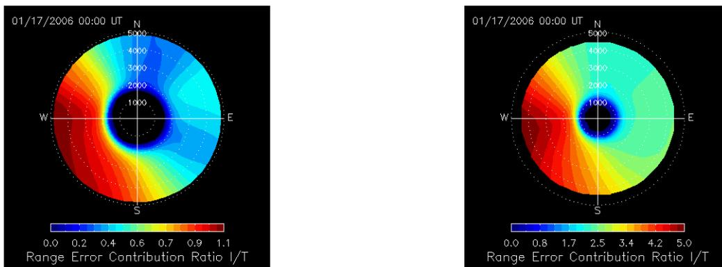
Fig. 4. The ratio of the ionospheric to tropospheric contributions to range error at 1° elevation (left panel) and at 10° elevation (right panel). Above 10° elevation the ionosphere dominates the range error except at very small ranges (when the target is below the ionosphere).
