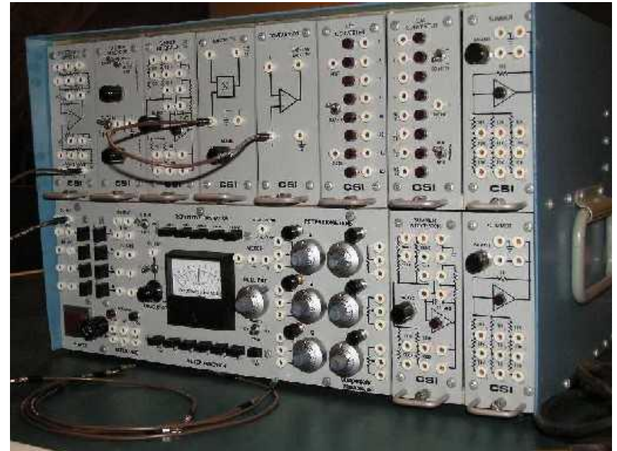
1970 Compumedic Analog Computer Model 6F13 Module
