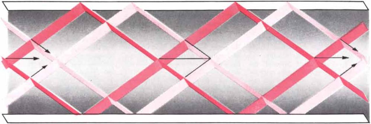
WAVE FRONTS (colored bands) advance through a wave guide by shuttling from wall to wall, in direction of slanted arrows, at
