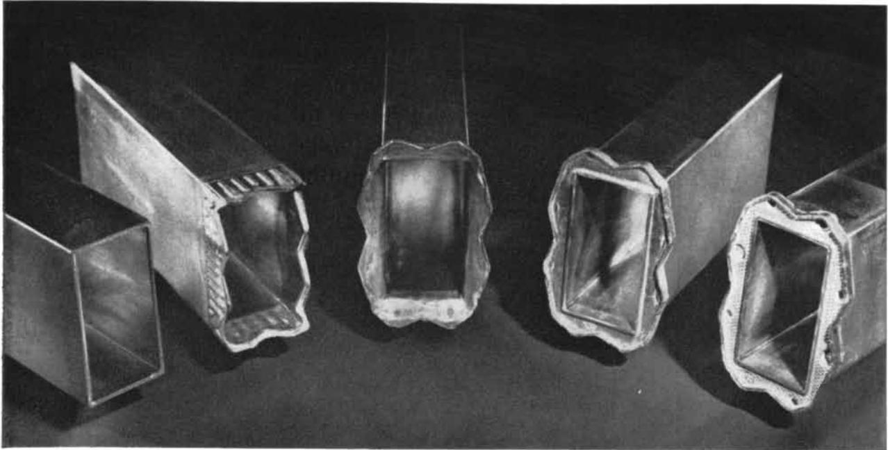
1 Waveguide cross-section before cold-flanging process.
