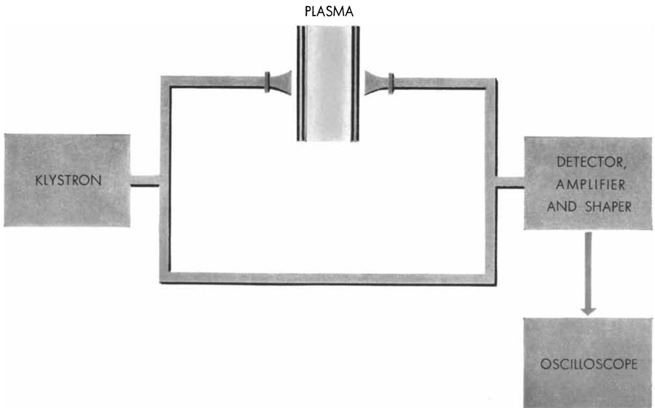
FREE-ELECTRON DENSITY in a plasma can be determined by measuring increase in speed of radio waves passing through the gas. Microwave output of klystron is split into two parts, one pass-
