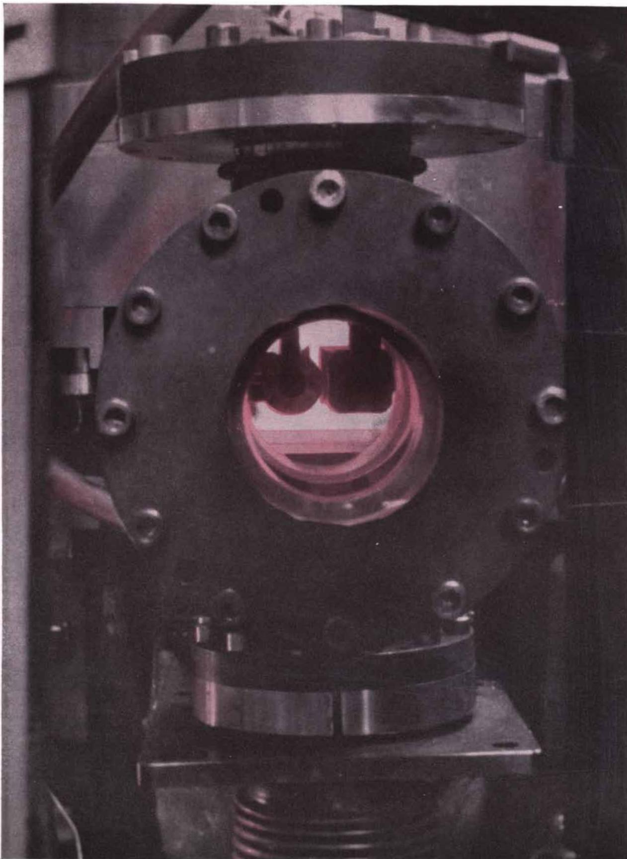
PLASMA, or highly ionized gas, which is producing the rosy glow in this photograph, is a medium in which radio waves have a phase velocity (*see text*) greater than  $c$  (the speed of light in a vacuum). The plasma is seen through a port in a Stellarator, a
