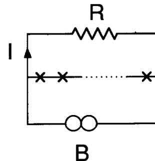
Fig. 1. Circuit schematic of a Josephson junction series array, subject to a parallel resistive load. Each cross represents a Josephson element.
